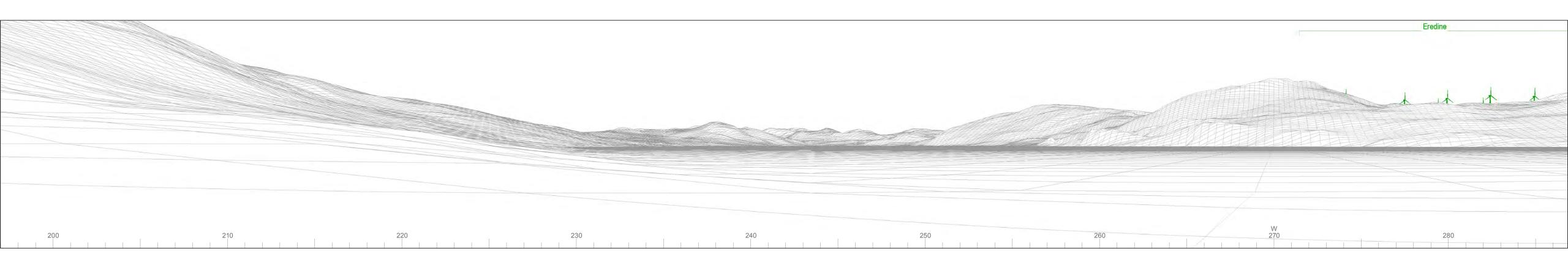
Wireline showing current proposed layout. 13 turbines @ 180m to blade tip height.
