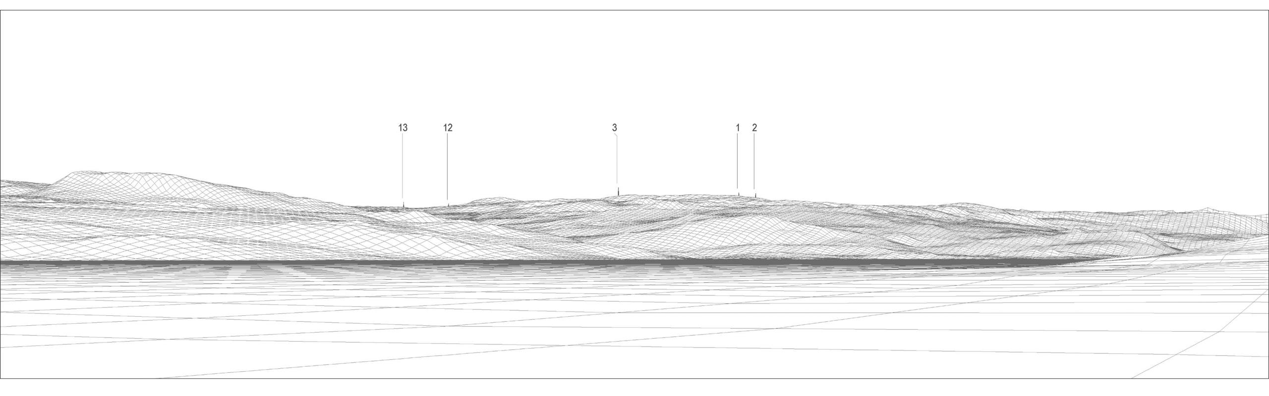
Wireline showing current proposed layout. 13 turbines @ 180m to blade tip height.
