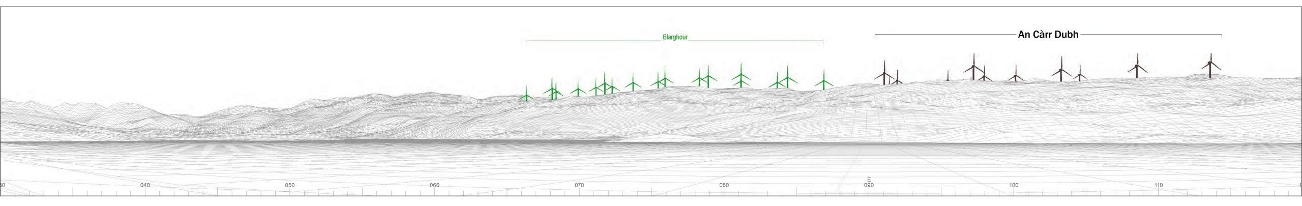
Wireline showing current proposed layout. 13 turbines @ 180m to blade tip height.
