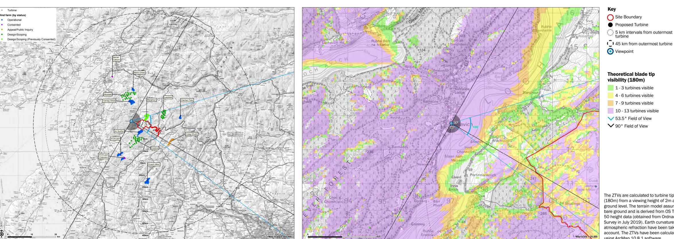
The ZTVs are calculated to turbine tip height (180m) from a viewing height of 2m above ground level. The terrain model assumes bare ground and is derived from OS Terrain 50 height data (obtained from Ordnance Survey in July 2019). Earth curvature and atmospheric refraction have been taken into account. The ZTVs have been calculated using ArcMap 10.8.1 software.
