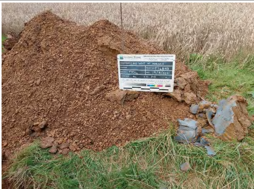
TP04 Stockpile showing clay
