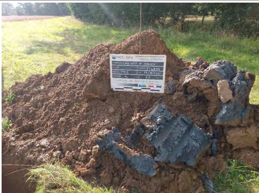
TP03 Stockpile showing clay
