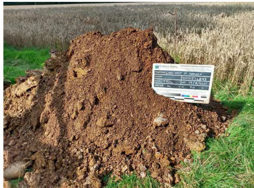
TP04 Stockpile showing gravels
