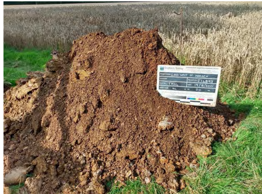
TP04 Stockpile showing gravels
