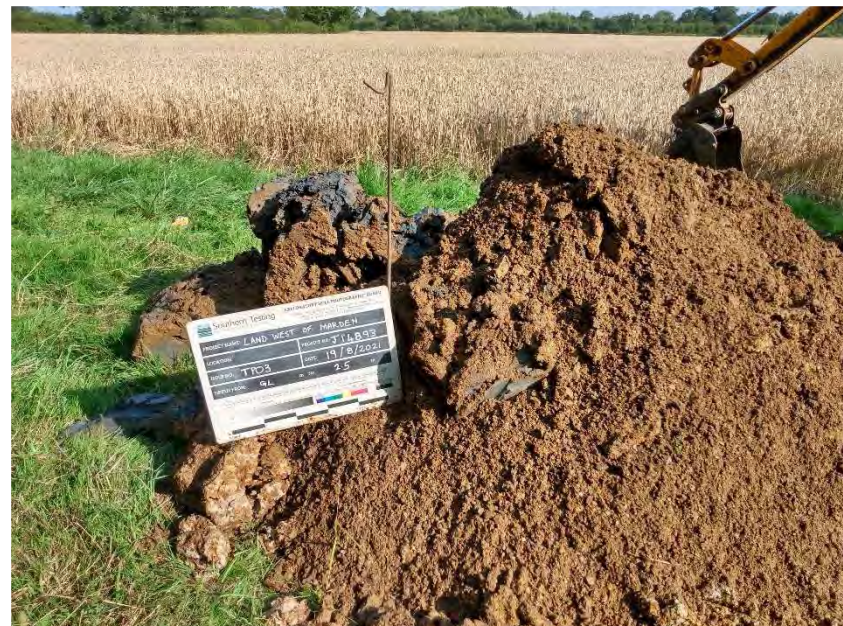
TP03 Stockpile showing gravels
