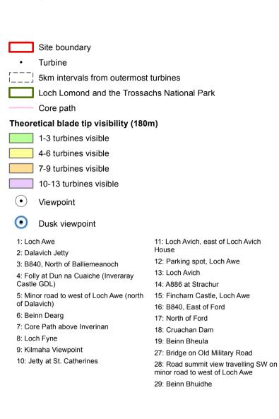
The ZTV is calculated to turbine tip height (180m) from a viewing height of 2m above ground level. The terrain model assumes bare ground and is derived from OS Terrain 50 height data (obtained from Ordnance Survey in July 2019). Earth curvature and atmospheric refraction have been taken into account. The ZTV was calculated using ArcMap 10.8.1 software.
