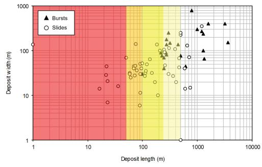
Plate 5.1 Runout distances for published peat landslides (after Mills, 2002), colours on the plot correspond to runout pathway zones on the left inset zoom Figure 7.4.9
