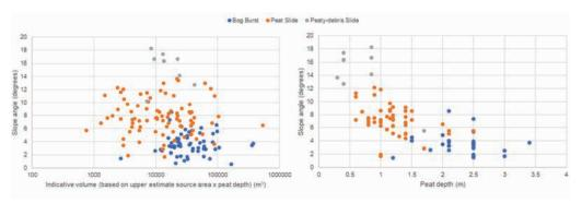
Plate 2.2 Reported slope angles and peat depths associated with peat slides and bog bursts (from literature review of locations, depths and slope angles, after Mills, 2002)
