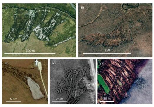
Plate 2.1 Characteristic peat landslide types in UK and Irish peat uplands: Top row - natural failures: i) multiple peat slides with displaced slabs and exposed substrate, ii) retrogressive bog burst with peat retained within the failed area; Bottom row - failures possibly induced by human activity: iii) peat slide adjacent to turbine foundation, iv) spreading around foundation, v) spreading upslope of cutting
