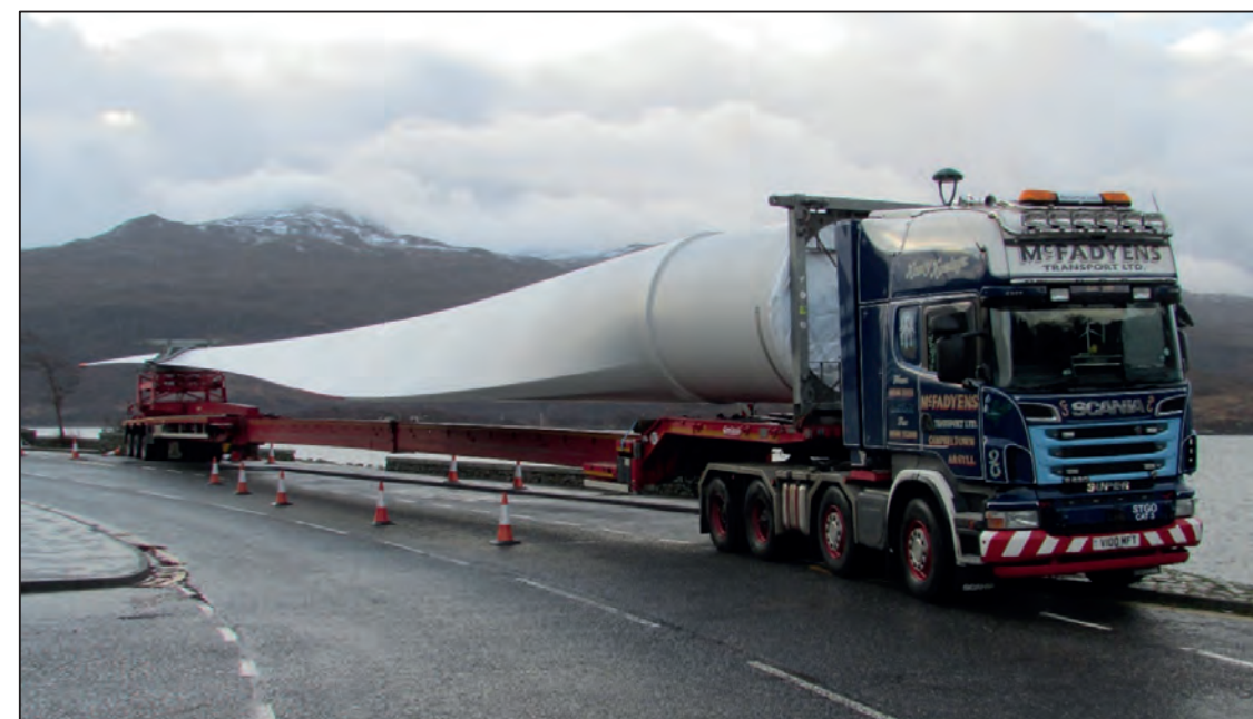
Figure 2: Super Wing Carrier with Loaded Turbine Blade
