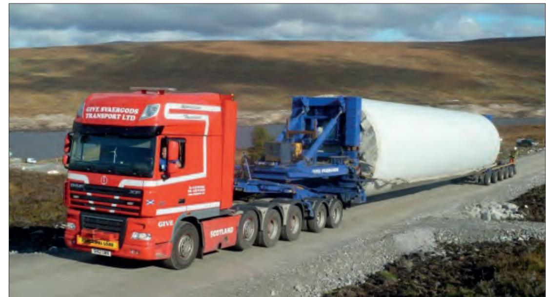
Figure 3 Typical Tower Transport Trailer
