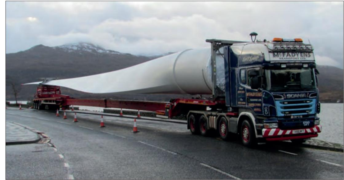
Figure 2 Super Wing Carrier with Loaded Turbine Blade
