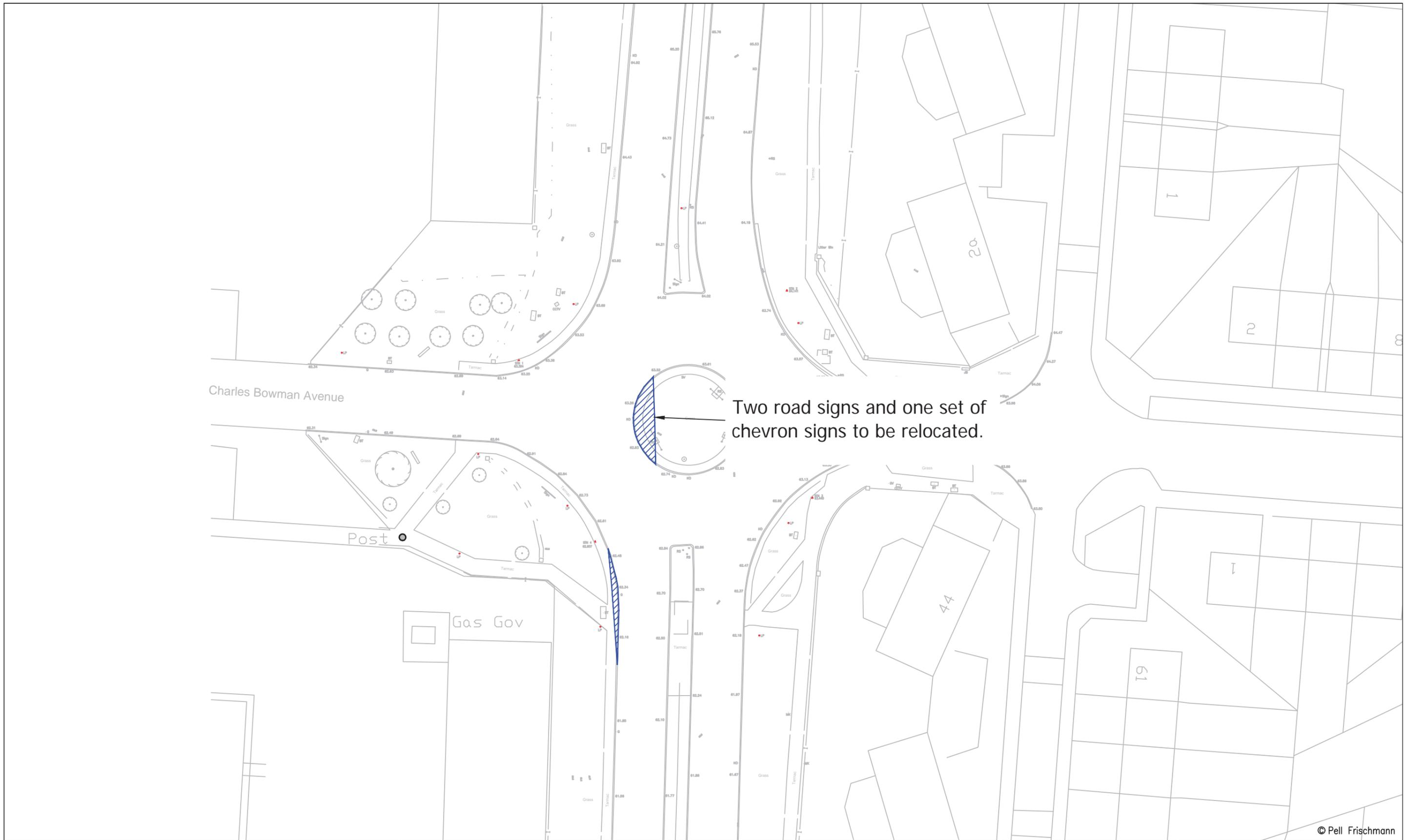
Two road signs and one set of chevron signs to be relocated.
