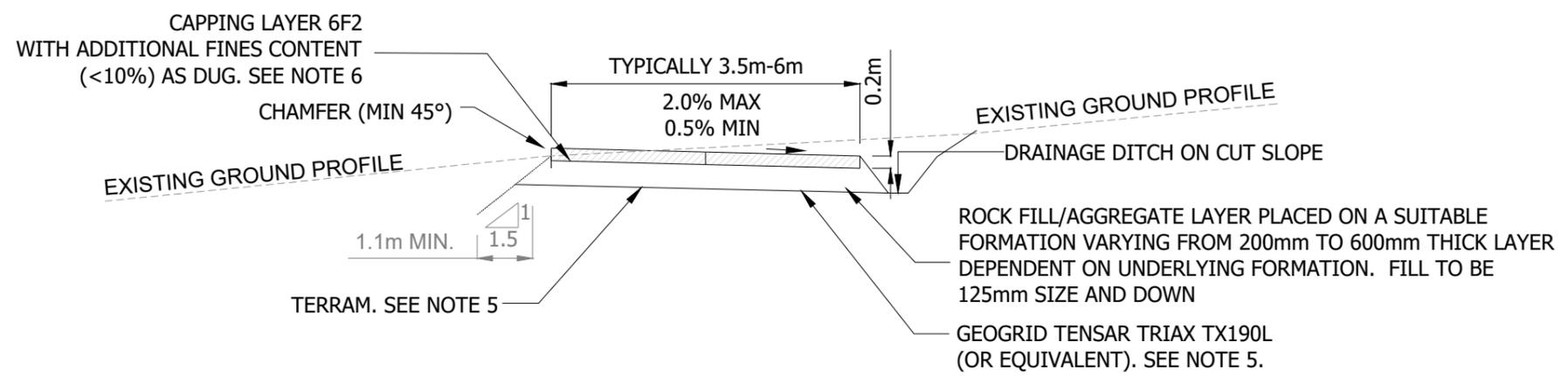
TYPICAL SECTION THROUGH EXCAVATED TRACK
